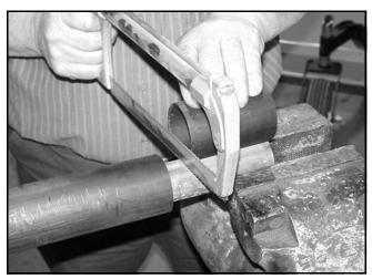
Figure 6. Cut Shaft to Length
